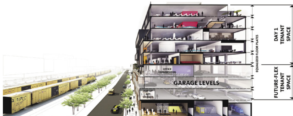
Giambrocco, a mixed-use project in Denver, includes three floors of flexible garage space that can be converted into office space. Credit: Gensler
