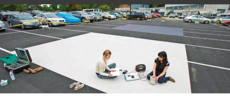
Researchers with the Lawrence Berkeley National Laboratory Heat Island Group use a reflectometer to take measurements of solar-reflective pavement coatings at the lab's California facility. Credit: Roy Kaltschmidt/Berkeley Lab, ©The Regents of the University of California, Lawrence Berkeley National Laboratory.
