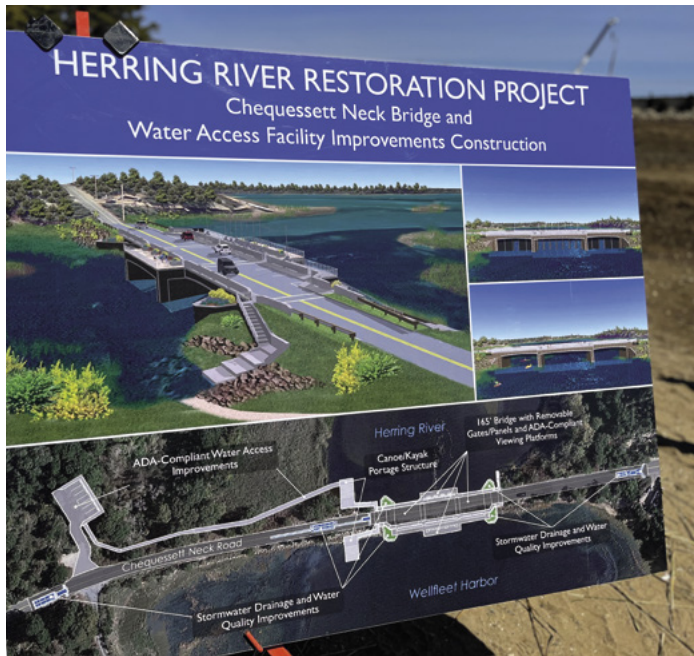
The Herring River Restoration Project in Wellfleet, Massachusetts, will return 677 acres of freshwater wetland to salt marsh by installing a new bridge with tide gates (left); the work has included collecting soil samples to analyze sediments, which can reveal information about the marsh's age and health (right). Credits (l-r): USGS Photo/Sara Ernst, NPS Photo/Kristina Vinduska.
