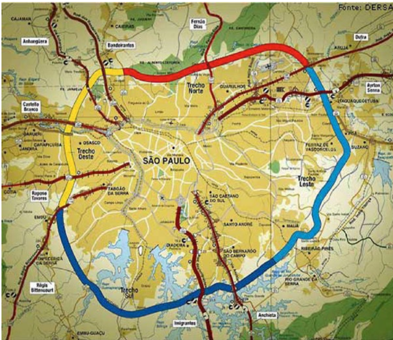
FIGURE 5 EXPROPRIATED REGION FOR THE NORTHERN SECTION OF THE RODOANEL, A ROAD THAT WILL ENIRCLE THE CITY OF SÃO PAULO
