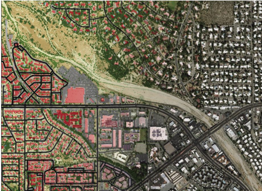
Chesapeake Conservancy's high-resolution land cover data—shown here beside the source imagery used to produce it—accurately depicts small features across the landscape. This level of detail is critical for planning projects that work with individual properties and landowners. Credit: Conservation Innovation Center
