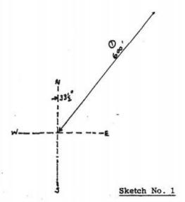
With a protractor lay off an angle of 33½ degrees East of North from the intersection of the North-South and East-West lines and extend this line, using a suitable scale, a distance of 600 feet.
