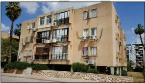
**The project is carried out in the non-demolition track and includes:** Reinforcement and renovation of the building; Addition of an elevator; Addition of 12 sqm to each existing flat; Adding 4 flats on the ground floor. Addition of 10 flats in 2.5 extra floors to be added to the building.
