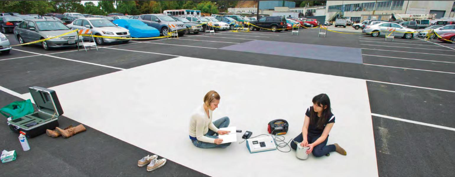
Researchers with the Lawrence Berkeley National Laboratory Heat Island Group use a reflectometer to take measurements of solar-reflective pavement coatings at the lab's California facility. Credit: Roy Kaltschmidt/Berkeley Lab, ©The Regents of the University of California, Lawrence Berkeley National Laboratory.
