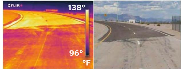
Thermal imaging reveals a dramatic temperature difference between light-colored pavement (foreground) and dark pavement (background) in Mesa, Arizona. Credit: Larry Scofield, APCA.
