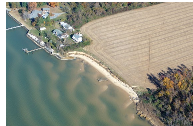
Unbuffered landscapes, such as this shoreline along the Chesapeake Bay, offer no protection from waves, leading to increased erosion, and can be a significant source of sediment and nutrient pollution. Credit: Jeff Allenby/ Chesapeake Conservancy
