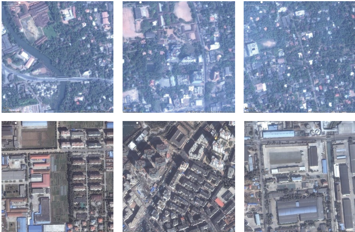
This image shows clear qualitative differences in the layouts of streets and blocks in the expansion areas of Kozhikode (top), which were mostly unplanned, and Qingdao (bottom), which were mostly planned. From 1990 to 2014, 28 percent of Qingdao's built-up area was in roads and streets compared to 8 percent in Kozhikode; four-way intersection and average block size were 51 square kilometers and 4.7 hectares respectively in Qingdao compared to 10 square kilometers and 7.5 hectares in Kozhikode; and the amount of residential development in formal land subdivisions or housing projects accounted for 76 percent of Qingdao's expansion area compared to 1 percent in Kozhikode. Credit: Bing
